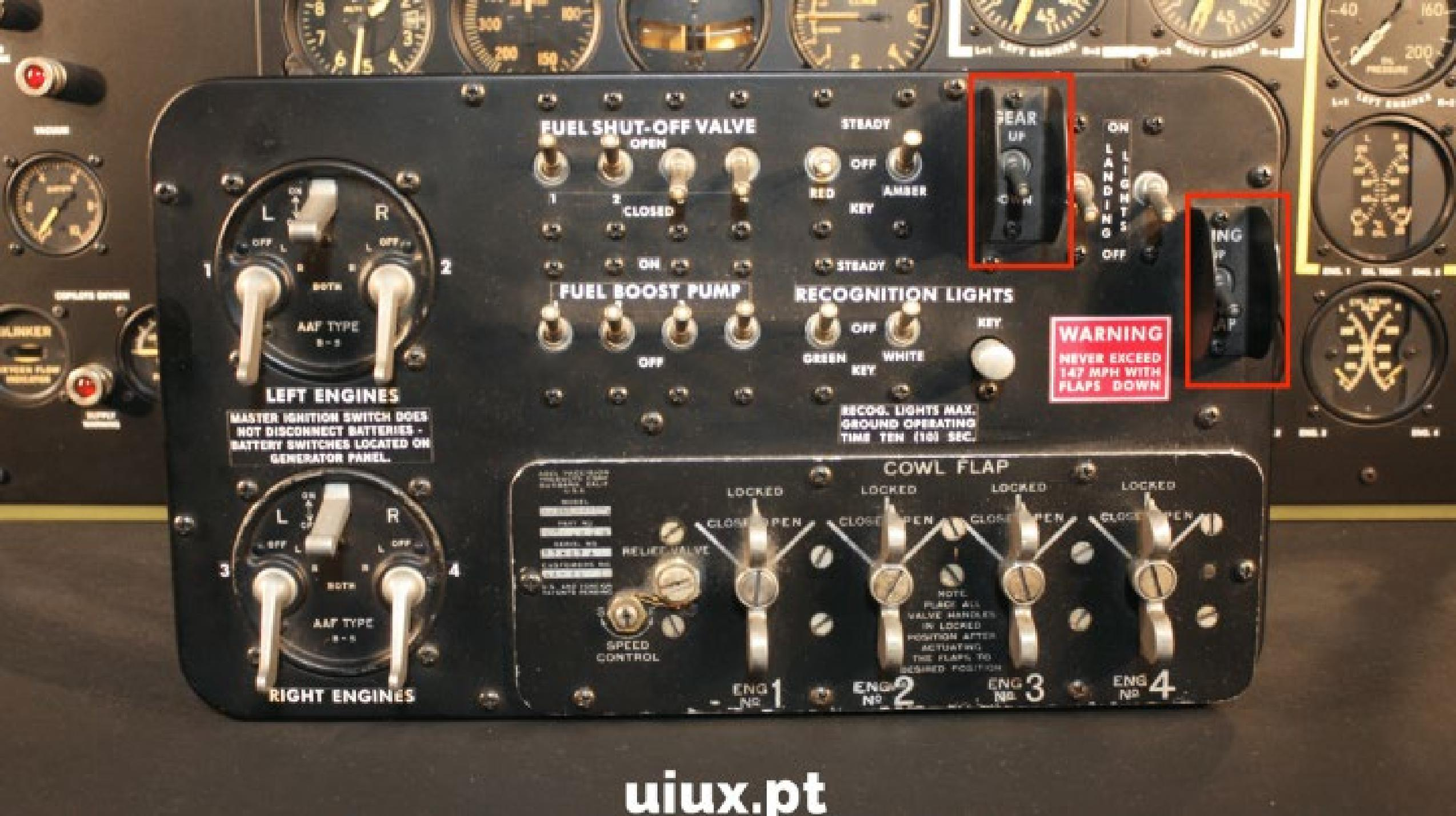
MASTER IGNITION SWITCH DOES NOT DISCONNECT BATTERIES - BATTERY SWITCHES LOCATED ON GENERATOR PANEL.
